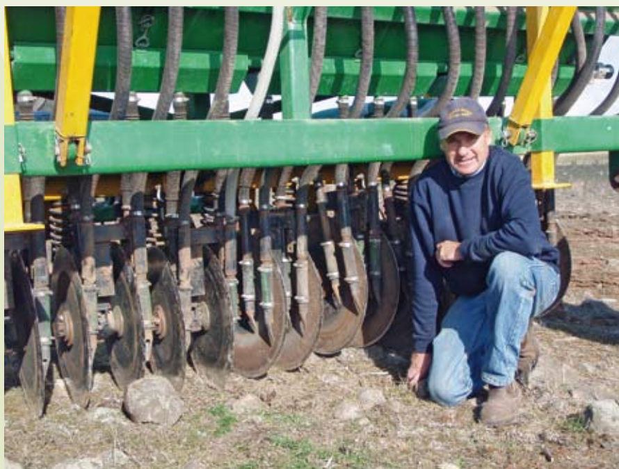
Philip uses a rock hopper disc seeder to establish perennial pastures after spraying in Chatsbury’s rockier tussock-filled paddocks.
